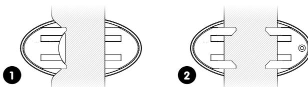
1. Slide one edge of the strap under one side of the H-clip on the back of the eClip.
